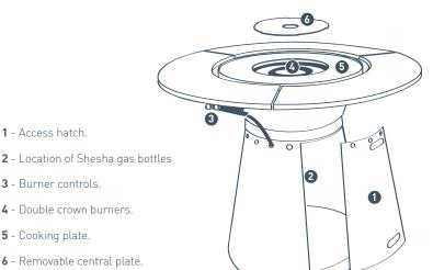
Remove the access hatch and open the gas inlet on the regulator. Remove the removable central plate to gain access to the burners. Open the burner controls and light them with a flame. Replace the centre plate and access hatch.
